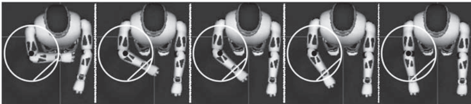
Fig. 8. Referring to figure 4, this is a sequence of snapshots for the movement at step 6 in the Laban score of figure 4. The free end of the right arm moves along a straight line between the starting position to the final one. Hence, the elbow (red point) does not remain at a fixed position in space. This makes the difference with the original motion performed by Naoko.
